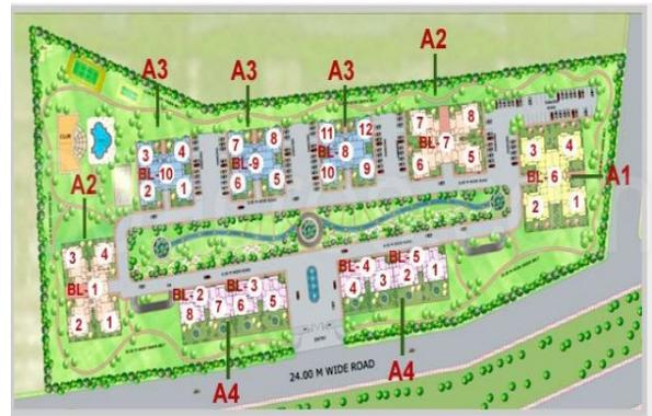
Fig. 23. Site Plan of Purvanchal height showing the tower spacing for free airflow [46].
