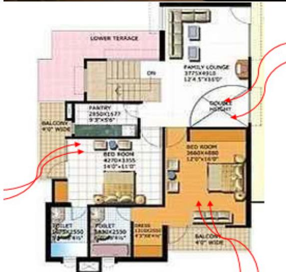
Fig. 22. Natural ventilation strategy in Purvanchal Height. (Source: Field Work, 2020).
